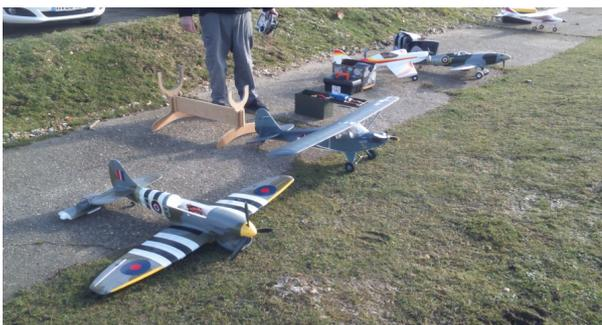
my new F3A competition aerobatic plane - an AJ Accuity 2 metre plane using the well tested 10s batteries (42 volts) with 5000mAh capacity. It runs a 21x13 prop and gives a 10 minute flight, long enough for the new P-19 FAI schedule.
